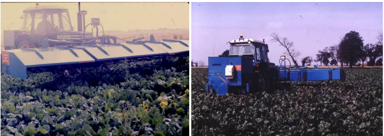
Figure 1. British Sugar Corp electrothermal weeder developed by Dr Mike Diprose in the 1970s and 1980s. Photos Dr Mike Diprose.
