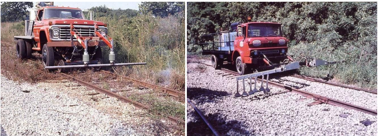
Figure 4. Railway weeding system. Photos Lasco via Dr Mike Diprose.
