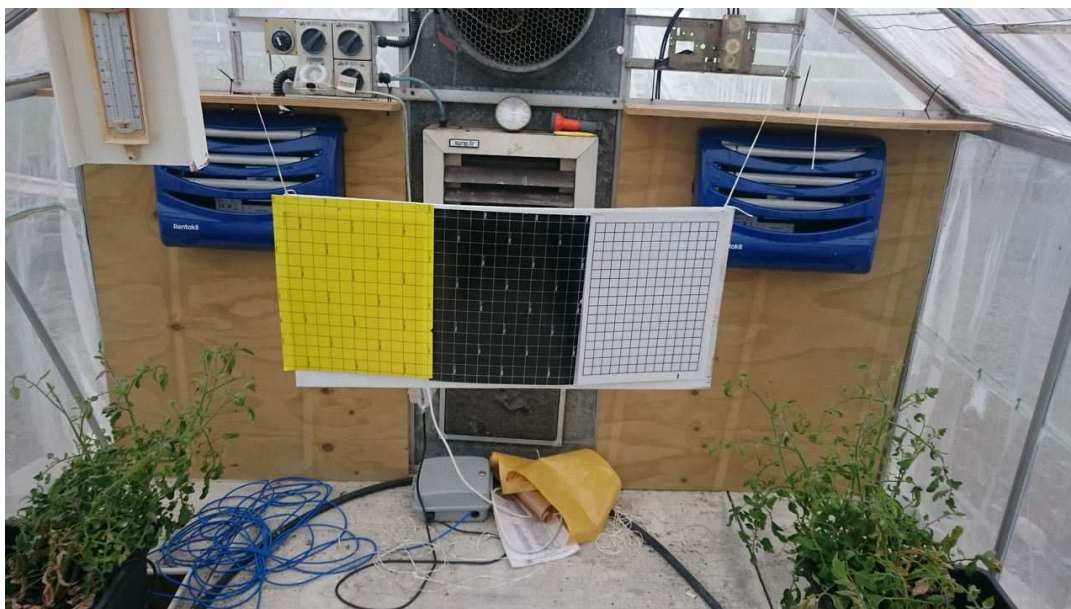
Figure 6. Experimental setup for comparing the relative attractiveness to TPP of the different coloured glue boards.
