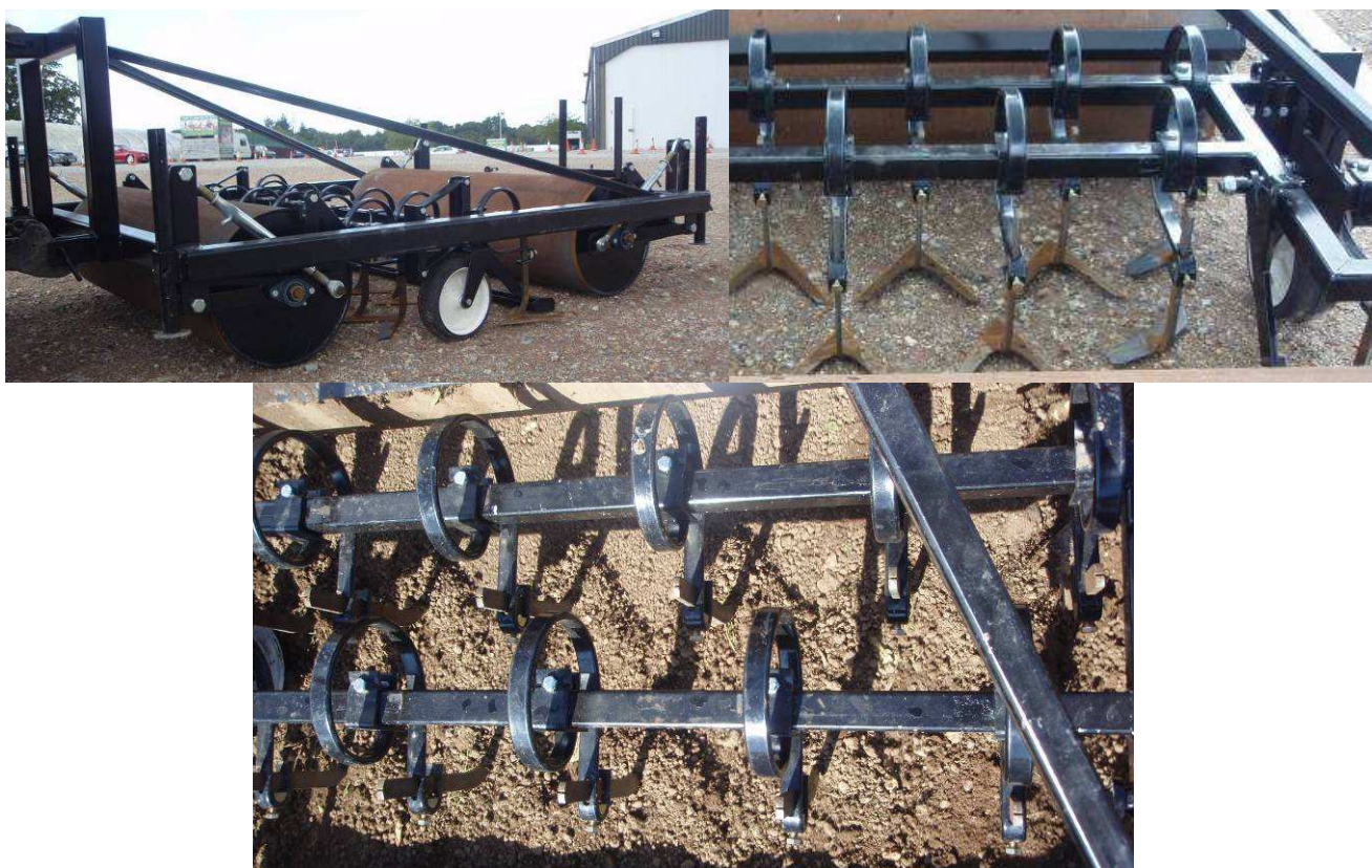
Figure 3. False seedbed tiller, capable of 100% kill of small weed seedlings (e.g., less than six true leaves) across the whole cropping soil surface while consistently penetrating only approx. one centimetre deep. © copyright Steam Weeding Ltd 2009.
