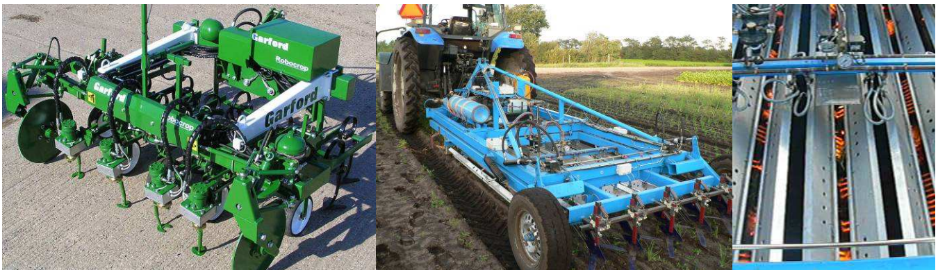
Figure 6. Two discriminatory intrarow weeders, Garford (left) using rotating hoes, Frank Poulsen (center and right) using micro-flames. Center and right photos © copyright Frank Poulsen Engineering ApS.
