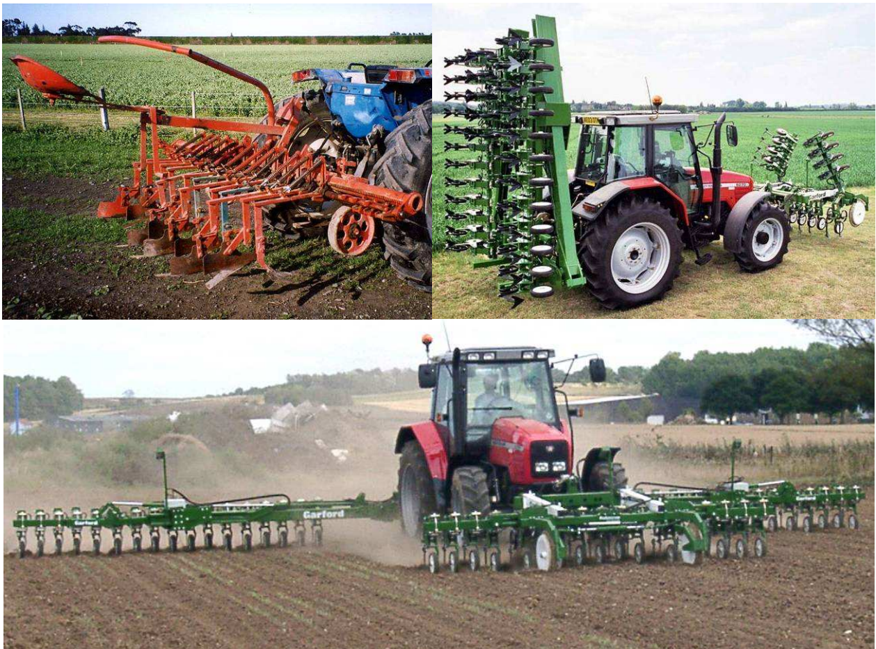
Figure 4. Pre-herbicide era Nicholson Webb interrow hoe (left) contemporary, multi-section folding interrow hoe (right and lower). Right and lower image © copyright Garford Farm Machinery Ltd 2010.
